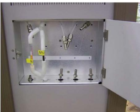
Ports can be used to support two parallel tubes each (sample and duplicate).
