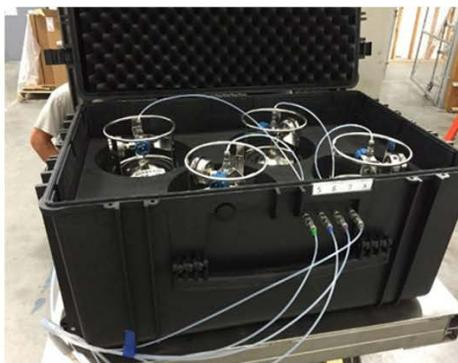
Rugged canister cases are loaded in the lab and sent into the field as a single unit.
